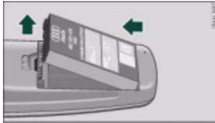
Fig. 25 Changing the battery
