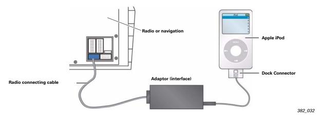
The Audi iPod adaptor can be used to connect the Apple iPod to radios with communication CAN bus. The adaptor converts the CD changer messages from the radio for the iPod. It can be connected as an alternative to the CD changer. Simultaneous operation of the CD changer and iPod adaptor is not possible, because both devices use the same port on the radio. All iPods with
