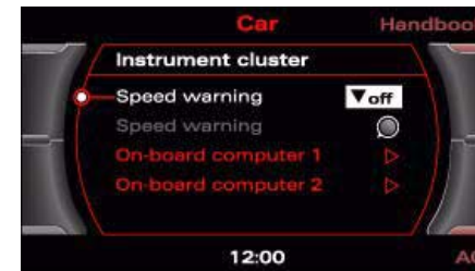
Fig. 23 Display: Setting speed limit warning 2
