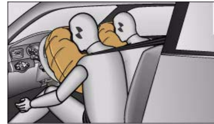
Fig. 216 Front airbags in inflated condition
