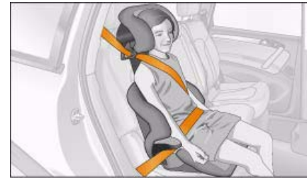
Fig. 228 A category 2/3 forward-facing child seat (with backrest) fitted on the rear seat
