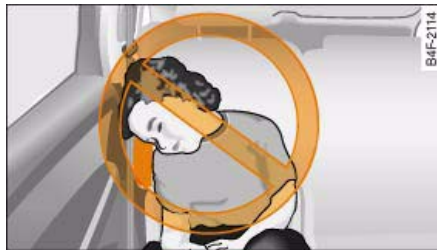
Fig. 224 Not properly restrained, and too close to the opening for the side airbag
