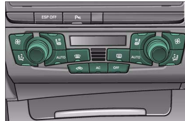
Fig. 112 Air conditioner controls
