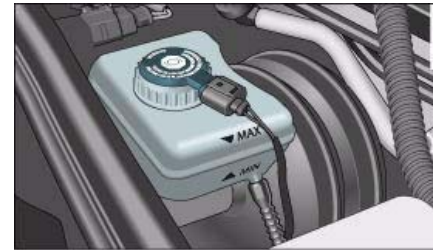
Fig. 258 Engine compartment: Markings on brake fluid reservoir
