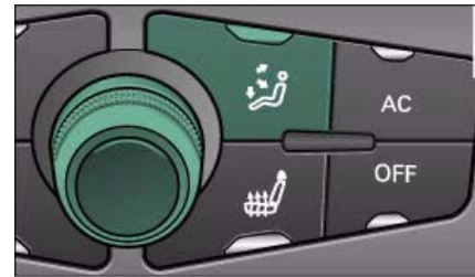
Fig. 108 Air distribution button and rotary control
