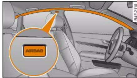
Fig. 220 Location of head-protection airbags above the doors
