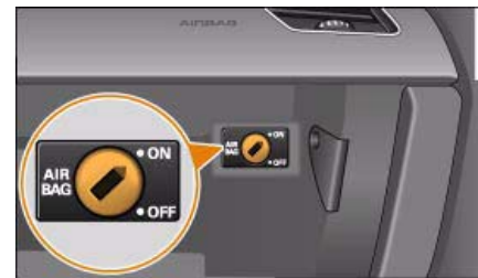
Fig. 222 Key-operated switch in glove box for deactivating front passenger's airbag ▶
