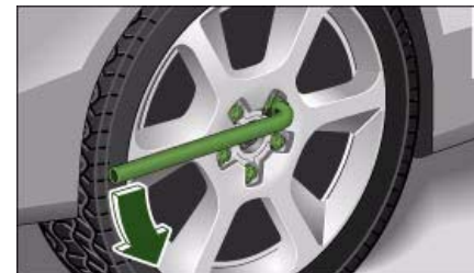
Fig. 272 Changing a wheel: Loosening wheel bolts
