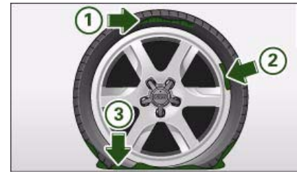
Fig. 269 The Tyre Mobility System is NOT suitable for repairing this type of damage to tyres.
