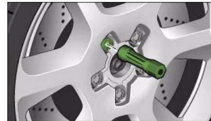
Fig. 275 Changing a wheel: Hexagonal socket in screwdriver handle to turn the wheel bolts after they have been loosened
