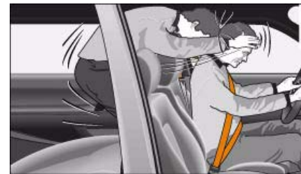
Fig. 207 A rear passenger not wearing a seat belt can be thrown forwards
