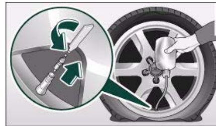
Fig. 270 Repairing a tyre
