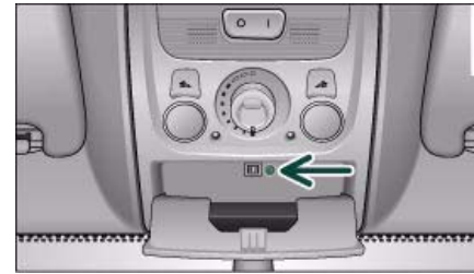
Fig. 52 Detail of headliner: Unscrewing the light housing
