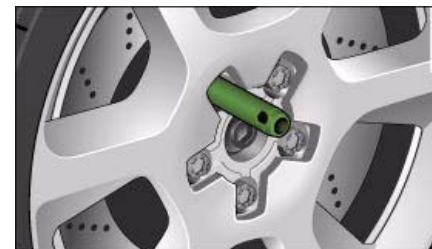
Fig. 276 Changing a wheel: Mounting pin in wheel bolt hole nearest to the top
