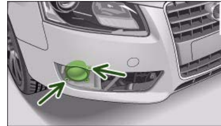
Fig. 299 Screws securing fog light
