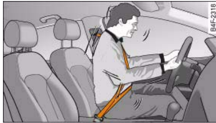
Fig. 203 Driver protected by the properly worn seat belt during a sudden brake manoeuvre
