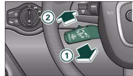
Fig. 141 Control lever for: Switching off the system (with speed memory function) and reactivating it
