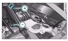
Fig. 259 Engine compartment: Terminals for jump leads and battery charger
