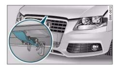
Fig. 251 Release catch under the bonnet
