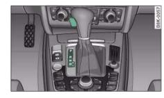
Fig. 177 Detail of the centre console: Selector lever with interlock button
