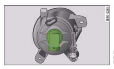
Fig. 300 Front fog light: Bulb holder is highlighted
