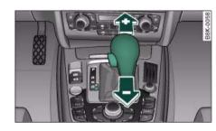
Fig. 180 Centre console: Manual gear selection (tiptronic mode)
