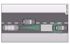
Fig. 151 The vehicle in front is outside the range of the radar sensor
