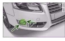
Fig. 299 Screws securing fog light
