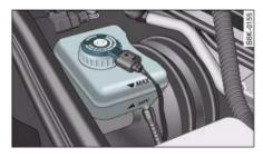
Fig. 258 Engine compartment: Markings on brake fluid reservoir
