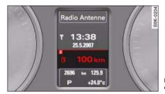
Fig. 17 On-board computer: Fuel range
