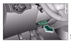
Fig. 129 Lever beneath steering column
