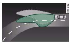
Fig. 59 adaptive light when driving
