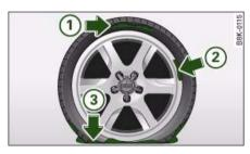
Fig. 269 The Tyre Mobility System is NOT suitable for repairing this type of damage to
