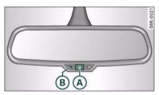
Fig. 71 Anti-dazzle interior mirror: On/off button with indicator lamp
