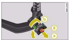
Fig. 243 Removable towing bracket: Removing the ball joint
