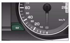
Fig. 6 Instrument cluster: Reset button
