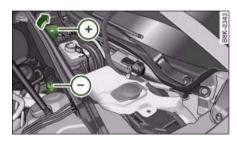
Fig. 278 Engine compartment: Terminals for jump leads and battery charger
