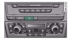
Fig. 185 Centre console: Parking aid switch
