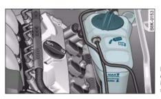
Fig. 257 Engine compartment: Markings on radiator expansion tank
