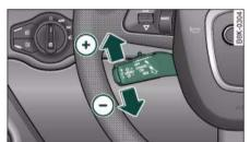
Fig. 140 Control lever for: Setting a new speed
