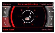
Fig. 127 Display: Seat heating
