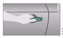
Fig. 39 Audi advanced key: Unlocking one of the doors
