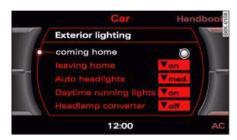
Fig. 56 Display: Exterior lighting
