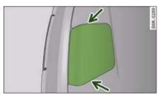
Fig. 307 Boot lid: Opening the cover in the boot lid
