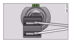
Fig. 292 Bulb with connector: The lug on the base of the bulb is highlighted
