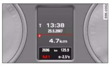
Fig. 181 Display: Manual gear selection (tiptronic mode)
