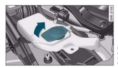
Fig. 260 Engine compartment: Windscreen washer container
