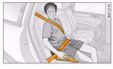
Fig. 229 A category 2/3 forward-facing child seat (without backrest) fitted on the rear seat
