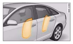
Fig. 219 Side airbags in inflated condition
