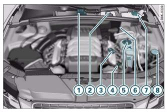
Fig. 252 Typical locations of fluid containers, engine oil dipstick and engine oil filler cap
