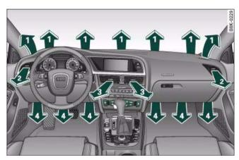
Fig. 110 Dashboard: Location of air outlets
