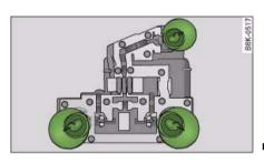
Fig. 309 Bulb carrier
