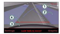
Fig. 194 MMI display: Blue area marking aligned in parking
