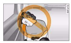
Fig. 224 Not properly restrained, and too close to the opening for the side airbag
