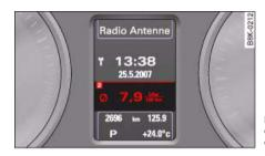
Fig. 18 On-board computer: Average fuel consumption
