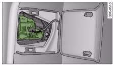
Fig. 308 Boot lid: Removing bulb carrier
