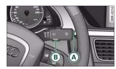
Fig. 20 Windscreen wiper lever: On-board computer controls
