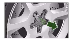
Fig. 271 Changing a wheel: Removing a hub
