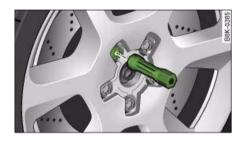
Fig. 275 Changing a wheel: Hexagonal socket in screwdriver handle to turn the wheel bolts after they have been loosened
