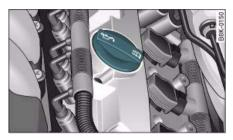
Fig. 256 Engine compartment: Engine oil filler cap
