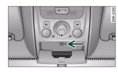
Fig. 52 Detail of headliner: Unscrewing the light housing
