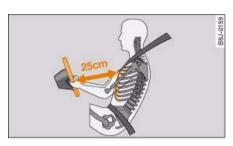
Fig. 217 Minimum distance from steering
