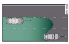
Fig. 172 Lanes of normal width are covered by the sensors
