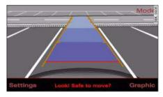
Fig. 193 MMI display: Aligning the vehicle
