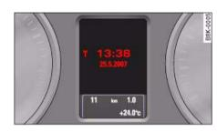
Fig. 4 Instrument cluster: Time and date display
