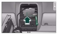
Fig. 53 Detail of headliner: Crank for manual operation
