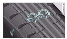
Fig. 262 Tyre tread: Tread wear indicators
