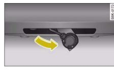
Fig. 244 Area below rear bumper: Folding up the socket
