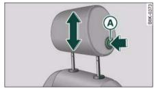
Fig. 79 Front seat: Adjusting head restraint
