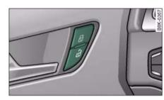
Fig. 41 Driver's door: Central locking switch
