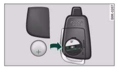
Fig. 126 Remote control: Changing battery
