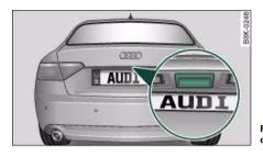
Fig. 46 Release catch on the boot lid
