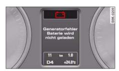
Fig. 25 Display: Symbol for serious malfunction
