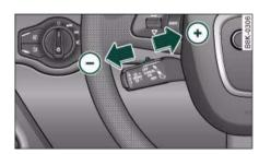
Fig. 142 Control lever for: Setting the distance
