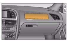
Fig. 215 Front passenger's airbag in dashboard
