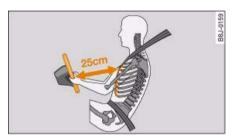
Fig. 199 Minimum distance between driver and steering
