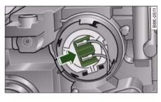
Fig. 291 Bulb holder for main beam head-
