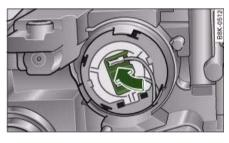
Fig. 297 Inserting bulb for dipped headlights
