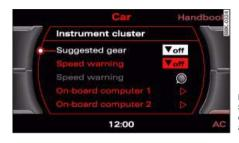
Fig. 12 Display: Switching the gear change indicator on and off
