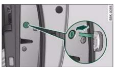
Fig. 44 Door: Locking the door manually
