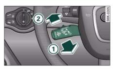
Fig. 141 Control lever for: Switching off the system (with speed memory function) and reactivating it
