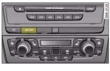
Fig. 233 Version B: Centre console (top), **ESP OFF button**
