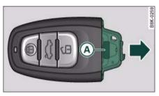
Fig. 33 Remote control key: Removing the battery carrier
