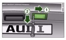
Fig. 310 Boot lid: Removing number plate light
