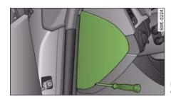
Fig. 283 Left side of dash panel: Fuse cover
