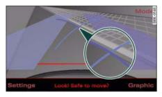
Fig. 195 MMI display: Blue marking touches edge of pavement
