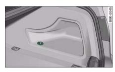
Fig. 98 Detail of the side trim in the luggage compartment: 12 Volt socket
