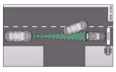
Fig. 155 Vehicle changing lane and vehicle stationary
