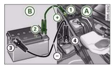
Fig. 279 Jumpstarting with the battery of another vehicle: A – Discharged battery, B – Boosting battery
