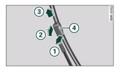
Fig. 70 Removing the wiper blades
