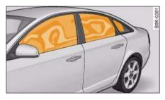
Fig. 221 Head-protection airbags in inflated condition
