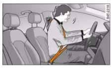
Fig. 203 Driver protected by the properly worn seat belt during a sudden brake manoeuvre
