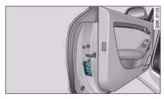
Fig. 261 Open driver's door (LHD vehicle) with sticker listing tyre inflation pressures
