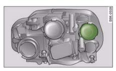
Fig. 290 Headlight unit: Rubber cap is highlighted
