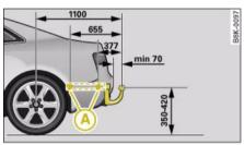
Fig. 245 Positions of securing points (side
