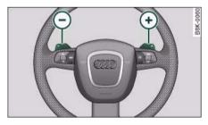
Fig. 182 Steering wheel: tiptronic switches
