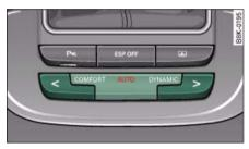
Fig. 174 Selector gate: **Control for Audi drive**
