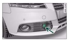
Fig. 136 Trim grille (front right): Position of radar sensor
