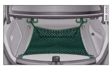
Fig. 85 Stretch net attached in position as retaining net
