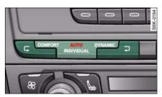
Fig. 175 Centre console: Control for Audi drive select
