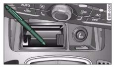
Fig. 184 Manual release of selector
