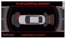
Fig. 186 Display: Graphical distance display
