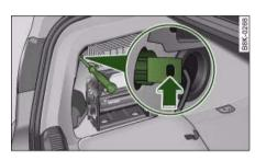
Fig. 302 Luggage compartment: Location of retaining screw for rear light
