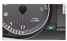
Fig. 22 Detail of the instrument cluster: SET button
