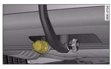
Fig. 242 Area below rear bumper: Electrical socket for trailer
