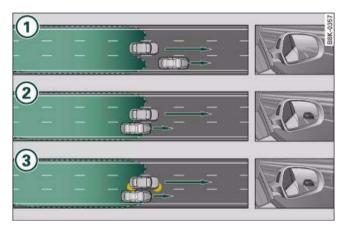
Fig. 170 side assist: Other vehicles being overtaken rapidly
