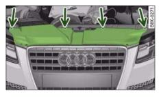
Fig. 288 Trim panel: Attachment points are marked by arrows
