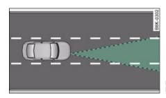
Fig. 137 Area covered by radar sensor
