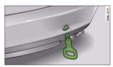
Fig. 282 Rear bumper: Fitting the towing eye
