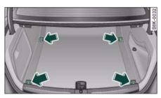
Fig. 83 Location of fastening rings in luggage compartment
