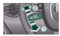
Fig. 138 Control lever for: Switching the system on and off
