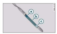
Fig. 253 Variant 1: Markings on oil dipstick
