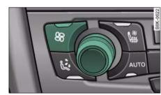
Fig. 115 Blower button and rotary control
