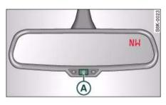
Fig. 73 Interior mirror: activated digital compass
