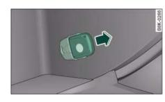
Fig. 36 Glove box: Adapter for spare key
