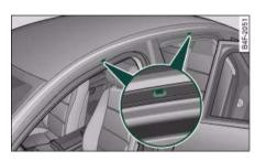
Fig. 92 Attachment points for carrier units
