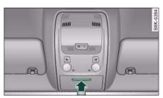
Fig. 102 Compartment for (sun)glasses in headliner
