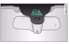
Fig. 159 Windscreen: Camera window for Audi lane assist
