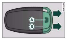
Fig. 34 Remote control key: Removing the emergency key
