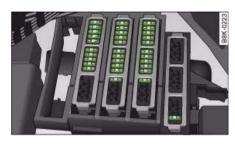
Fig. 286 Diagram of fuse panel
