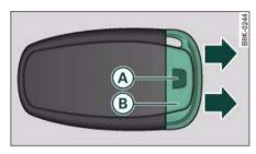
Fig. 32 Remote control kev: Removing the emergency key
