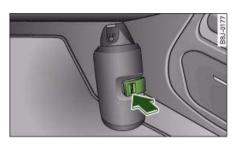
Fig. 266 Fire extinguisher in footwell on front passenger's side
