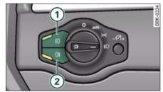
Fig. 55 Switch for front fog lights
