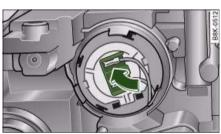
Fig. 293 Fitting bulb for main beam headlights
