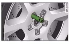
Fig. 276 Changing a wheel: Mounting pin in wheel bolt hole nearest to the top
