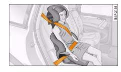
Fig. 228 A category 2/3 forward-facing child seat (with backrest) fitted on the rear
