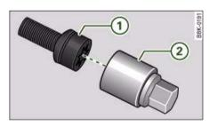
Fig. 277 Anti-theft wheel bolt with adapter
