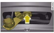
Fig. 240 Removable towing bracket: Inserting the ball joint
