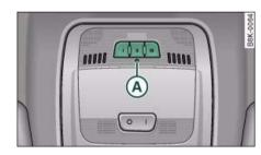
Fig. 197 Operating unit in headliner
