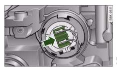
Fig. 295 Bulb holder for dipped headlights
