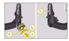
Fig. 239 Removable towing bracket: Setting the spring mechanism to the "ready" position
