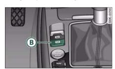
Fig. 133 Detail of the centre console: Button for Audi hold assist
