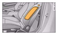
Fig. 218 Location of side airbag in driver's seat
