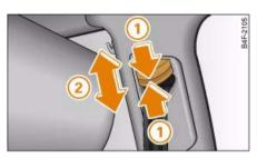
Fig. 212 Belt height adjustment for the front seats: guide
