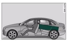
Fig. 82 Heavy items should be placed as far forwards as possible.
