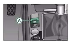
Fig. 132 Centre console: Parking brake
