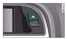
Fig. 60 Switch for hazard warning lights
