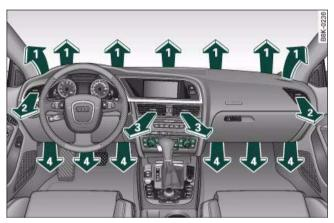
Fig. 119 Dashboard: Location of air outlets
