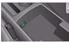
Fig. 99 Electrical socket in the centre console
