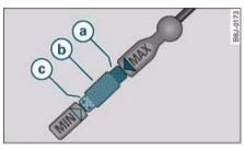
Fig. 254 Variant 2: Markings on oil dipstick
