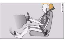
Fig. 200 Correct head restraint position for the driver
