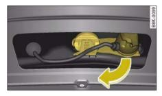
Fig. 236 Area below rear bumper: Folding down the socket
