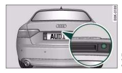
Fig. 191 Boot lid: Location of reversing camera
