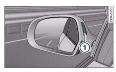
Fig. 164 Warning lamp on exterior mirror (driver's side)
