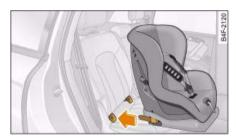
Fig. 231 The ISOFIX child safety seat is pushed into the protective sleeves.
