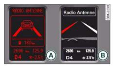
Fig. 160 Instrument cluster: lane assist switched on and in warning mode
