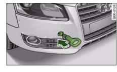
Fig. 281 Front bumper: Fitting the towing eye
