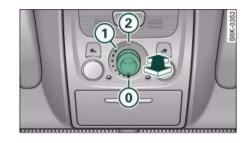
Fig. 51 Detail of headliner: Rotary control for sun roof
