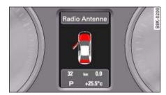
Fig. 14 Display: Door catches/boot lid warning
