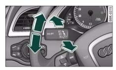
Fig. 61 Turn signal and main beam headlight
