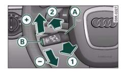
Fig. 134 Control lever and pushbutton
