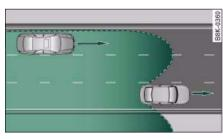
Fig. 173 Narrow lanes: side assist may react to vehicles travelling two lanes away
