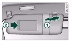
Fig. 64 Passenger's side: Sun visor
