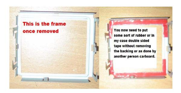
Once the foam is stuck down, don't remove the other backing as you don't want the frame to stick to the LCD display.
