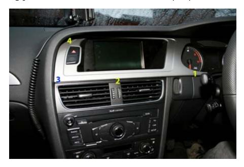
The positions of the clips on the rear of the trim is shown below:
