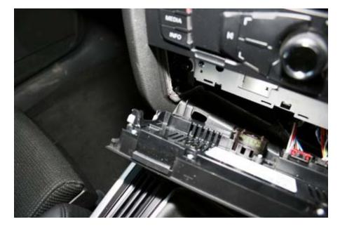
Pulling firmly towards you will unclip the panel. Only pull far enough to release the clips on the side your are working on, other wise you may snap off the clips on the other side. Repeat the operation for the other side of the climate control panel. The panel can be tipped forward and moved to the left to give access to the lower bolts of the Head Unit. Remember to protect the top of the ash tray with a cloth to prevent scratching.
