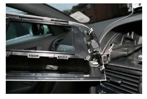
Once removed, this can easily be swung around and perched on top of the dashboard, out of the way, without the need to disconnect the Hazard warning switch / Airbag warning light harness.
